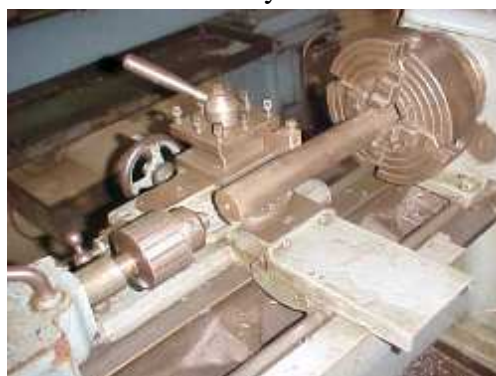
Fig. 2.24 Holding drill chuck and drill in tailstock
