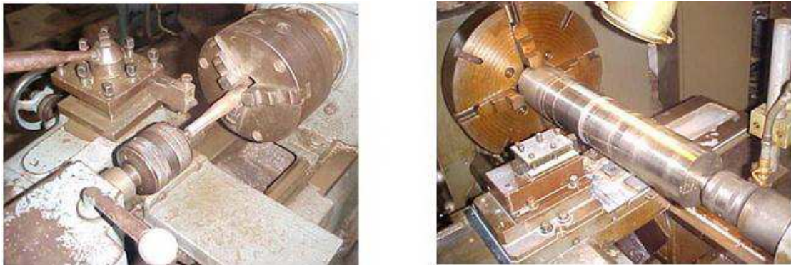
Fig. 2.19 Work held between chuck and revolving centre
