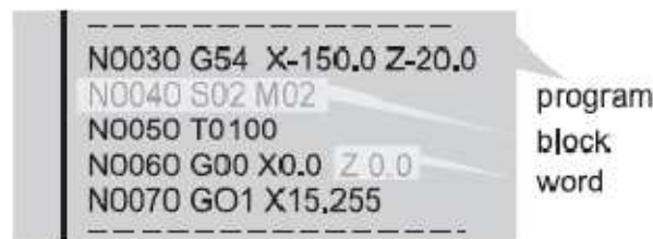
Structure of a NC program
