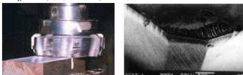
Fig. 1.49 (a) Schematic view of wear pattern of face milling insert
